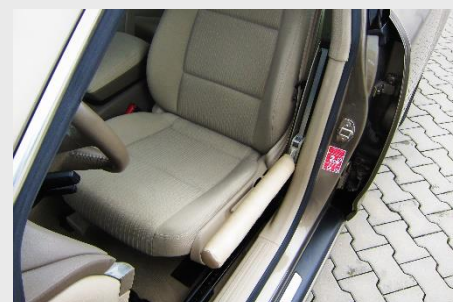
Application for lifting from seat to stand, AUDI A6.
